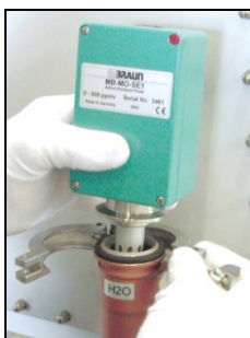
11. Insert measuring probe and re-clamp.
