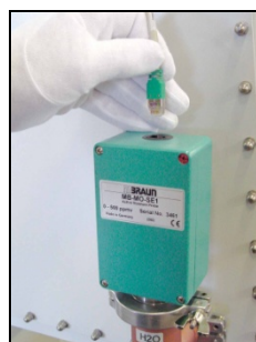
1. Disconnect plug connector.
