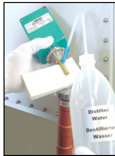
6. Moisten sensor with distilled water.
