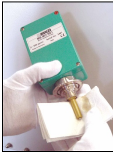
7. Carefully clean and dry winding.
