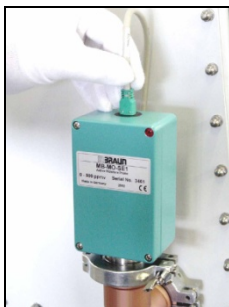
13. Insert plug connector.
