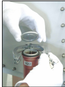
10. Remove clamp and dummy plug.
